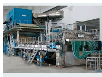
RECONSTITUTED TOBACCO MACHINE, WIDTH 2910 MM, SPEED 150 MPM, 90-200 GSM
