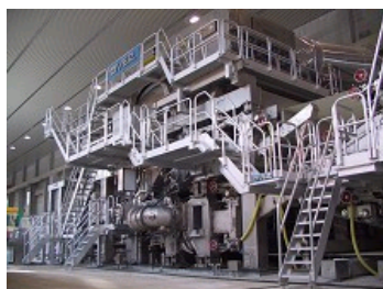
TISSUE MACHINE, WIDTH 2850 MM, SPEED 2000 M/MN, 120 T/J
