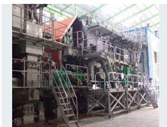
PAPER MACHINE, WIDTH 4510 MM, SPEED 1000 MPM, 125-200 GSM
