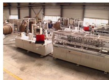
HIGH SPEED SPIRAL WINDING LINE FOR THE PRODUCTION OF CARDBOARD CAN BODIES
