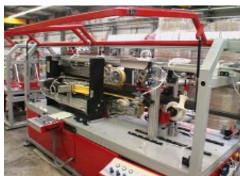
SIRPAK LINE FOR THE PRODUCTION OF ROUND AND NON-ROUND COMPOSITE CAN BODIES
