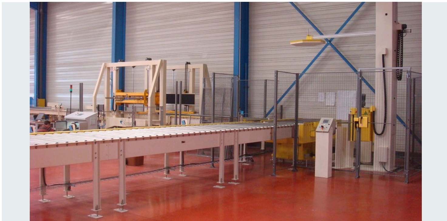
FULL TURNTABLE AUTOMATIC STRETCH WRAPPING SYSTEM, WITH LOAD STABILIZER AND APPLICATION OF THE TOP SHEET
