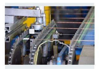
PRODUCTION OF FLAGGED TIG WIRES FOR THE AERONAUTICAL SECTOR
