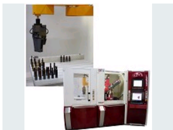
CA3+ WITH ROBOT FOR CHANGING TOOLS AND SLEEVES
