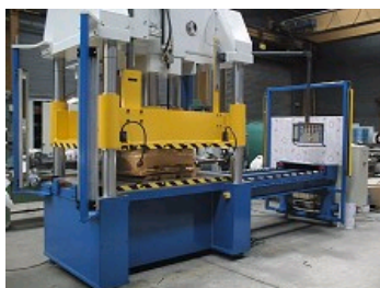
FORMING HYDRAULIC PRESS FOR AEROSPACE INDUSTRY
