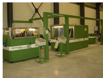
EXPANDED LEAD LINE FOR PRODUCTION OF SGRIDS FOR CAR BATTERIES MANUFACTURERS
