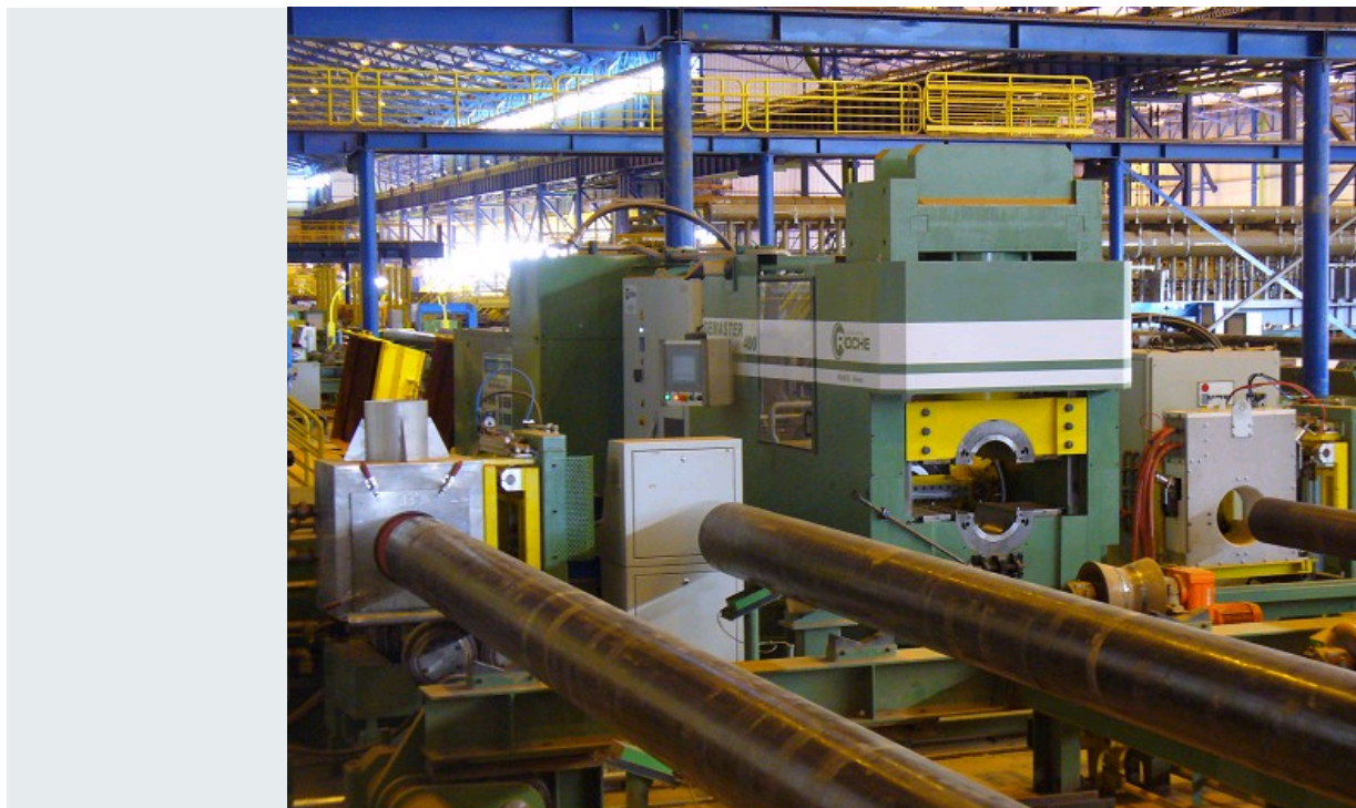
COMPLETE CALIBRATION / SWAGING CELL FOR OIL&GAS PIPES
