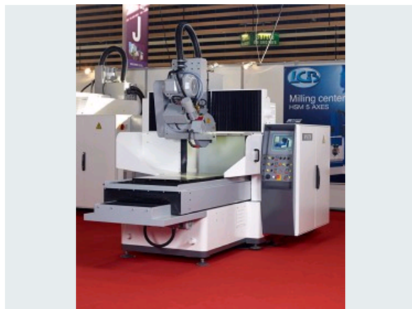
RN 1270 - PORTAL GRINDING MACHINE TRAVELS : 1200 X 700 X 450
