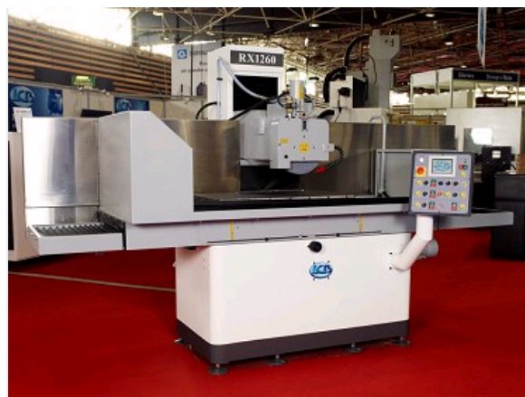
RN 1260 - SINGLE COLUMN GRINDING MACHINE TRAVELS : 1200 X 600 X 400
