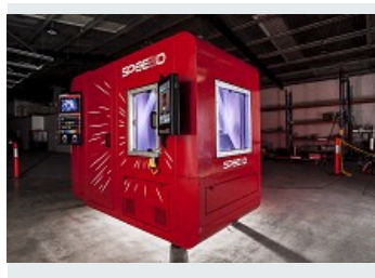
SPEED3D IS THE FIRST ADDITIVE MANUFACTURING TECHNOLOGY BASED ON THE COLDSPRAY PROCESS.
