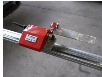
OPTION : DIGITAL READOUT OF THE STOP OF THE RULER
