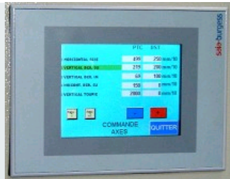
CNC CONTROLLER FOR AUTOMATIC POSITIONING OF THE TOOLS
