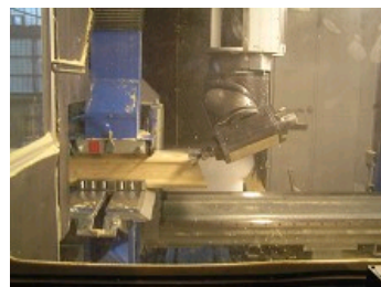
SPEEDER: 4 AXIS CNC MACHINING CENTER FOR ROOF AND TIMBER FRAME WALL ELEMENTS
