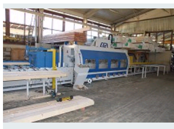
BRUSHWOOD C400: STRUCTURAL BRUSHING CENTER FOR SOLID & GLUED BEAMS, WOODEN HOUSES ELEMENTS AND CLADDINGS
