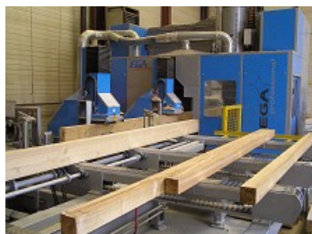
VEGA: 5 AXIS TIMBER MACHINING CENTER FOR WOODEN STRUCTURE AND ROOF ELEMENTS
