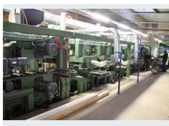
BRUSHWOOD X400: 8 FACES CNC BRUSHING LINE FOR SOLID & GLUED BEAMS WITH SIZE UP TO 400 X 400 X 14M
