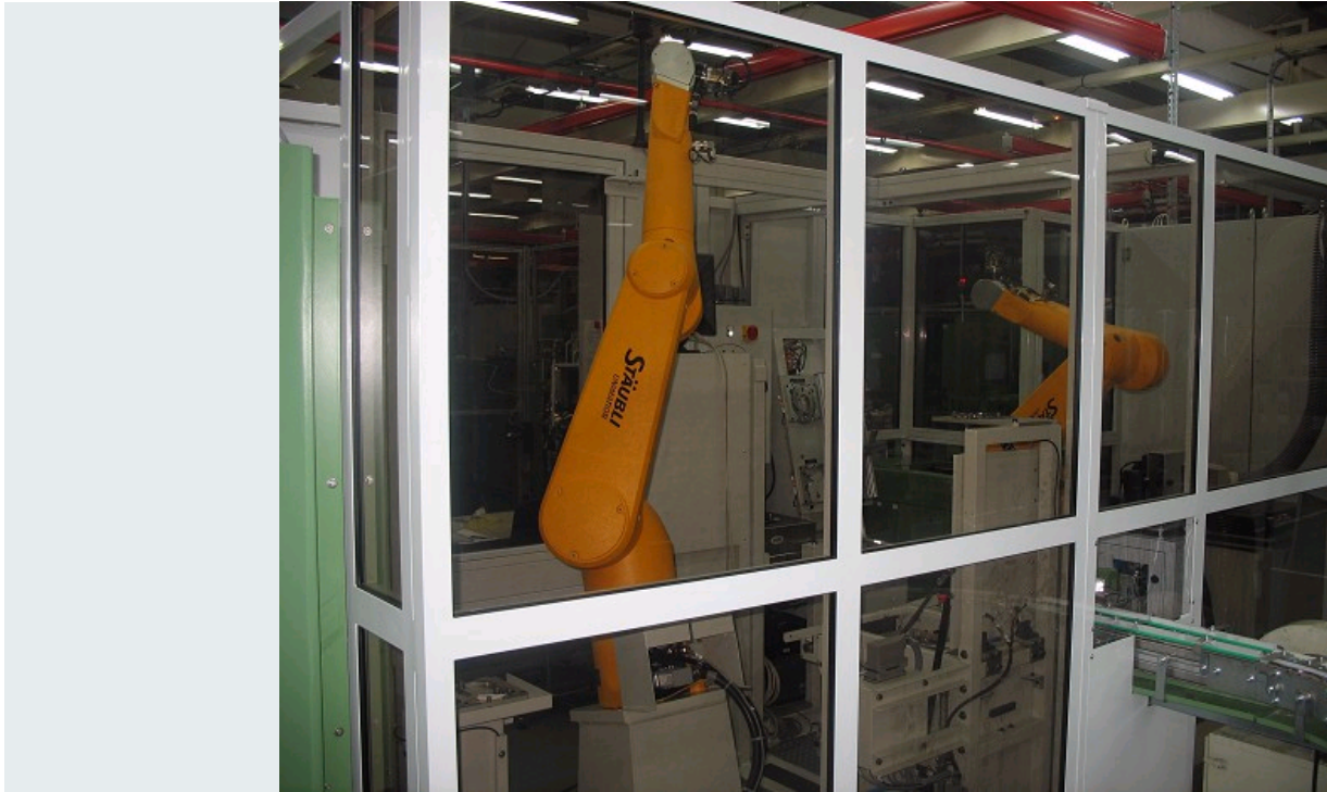
AUTOMATED LINE FOR MACHINING MECHANICAL PARTS COMPOSED BY 2 ROBOTS, FEEDING SYSTEM, CONTROL SYSTEM, DETECTION BY VISION SYSTEM, ROTATIVE TABLE, SAMPLE STATION AND PACKAGING
