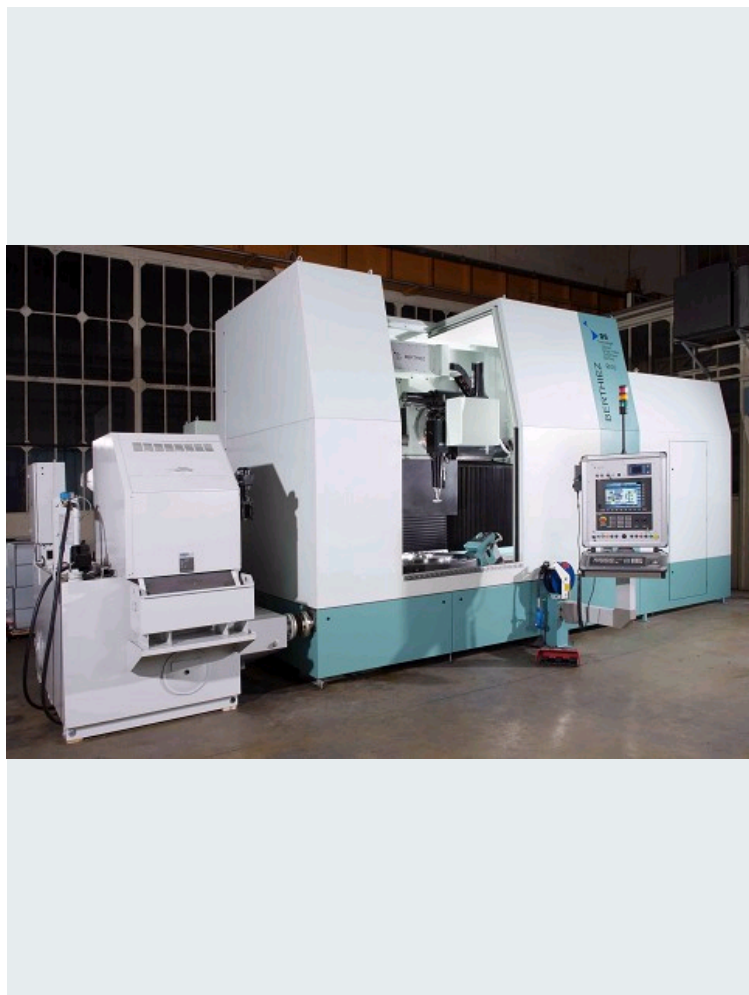
VERTICAL GRINDING MACHINE WITH TABLE DIAMETER 800 UP TO 6000 MM, HYDROSTATIC TABLE BEARING, DIRECT DRIVE BY TORQUE MOTOR, GRINDING SPINDLES WITH 7 UP TO 45 KW, HARD TURNING
