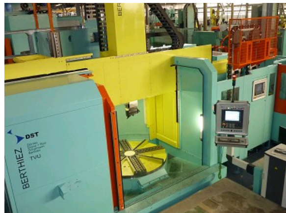
VERTICAL TURNING LATHES WITH TABLE DIAMETER 800 UP TO 2500 MM, HIGH PRESSURE COOLANT 400 BAR, TURNING, MILLING, GRINDING, PALLETIZATIONS
