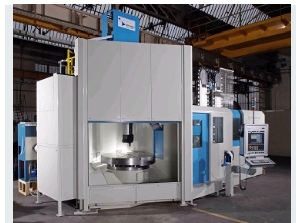
TVU 2000/160 HIGH PRESSURE COOLANT 400 BAR, CAPTO C8, TOOL CHAIN MAGAZINE 80 POCKETS, PALLETIZED PRODUCTIVITY GAIN UP TO 50%
