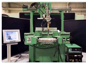
MULTISURFACER : AUTOMATED WELDING EQUIPMENT FOR HARDFACING
