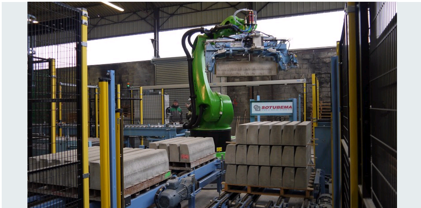
MULTI-AXIS ROBOTIC ISLAND EQUIPPED WITH A MULTIFUNCTION GRIPPER
