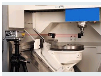
PITCH MEASURING WITH LASER INTERFEROMETER
