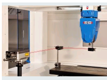
MEASURING ACCURACY WITH A LASER INTERFEROMETER
