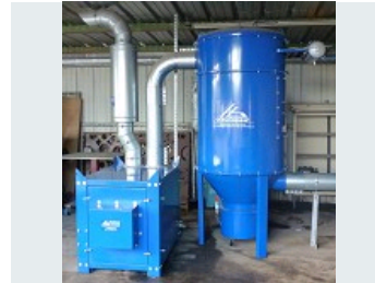
CENTRALIZED HIGH SUCTION UNIT
