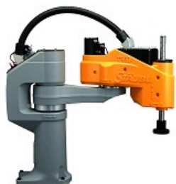
SCARA ROBOTS WITH REACH FROM 220 TO 800 MM, MAXIMUM PAYLOAD OF 8 KG
